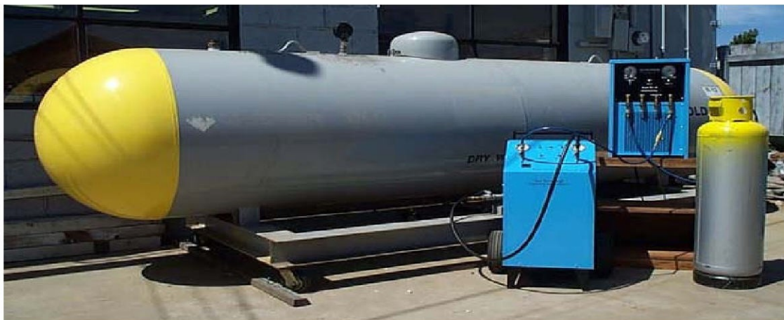
VS-29 Deep Vacuum System and RV-10 Recovery System Evacuating a 10,000 lb. / 4,545 kg Cylinder
